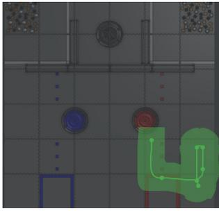
With the help of RoadRunner, programmers can design trajectories on a 2D plane of the field's plane. These trajectories can then be ran on the robot, with built-in error correction through the use of the built-in PID controller in the REV hub.
